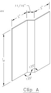
16g ASTM A653 Grade 33 G60 Bare metal thickness: t = 0.0538"
